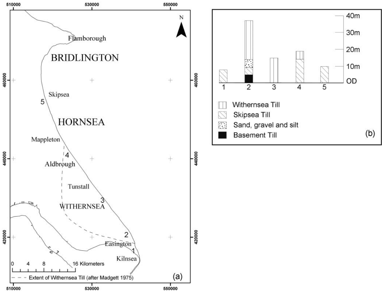
Fig. 2. (a) Plan view of the spatial distribution of the Withernsea Till, and (b) cliff face logs (after Catt & Madgett 1981; Berridge & Pattison 1994).
