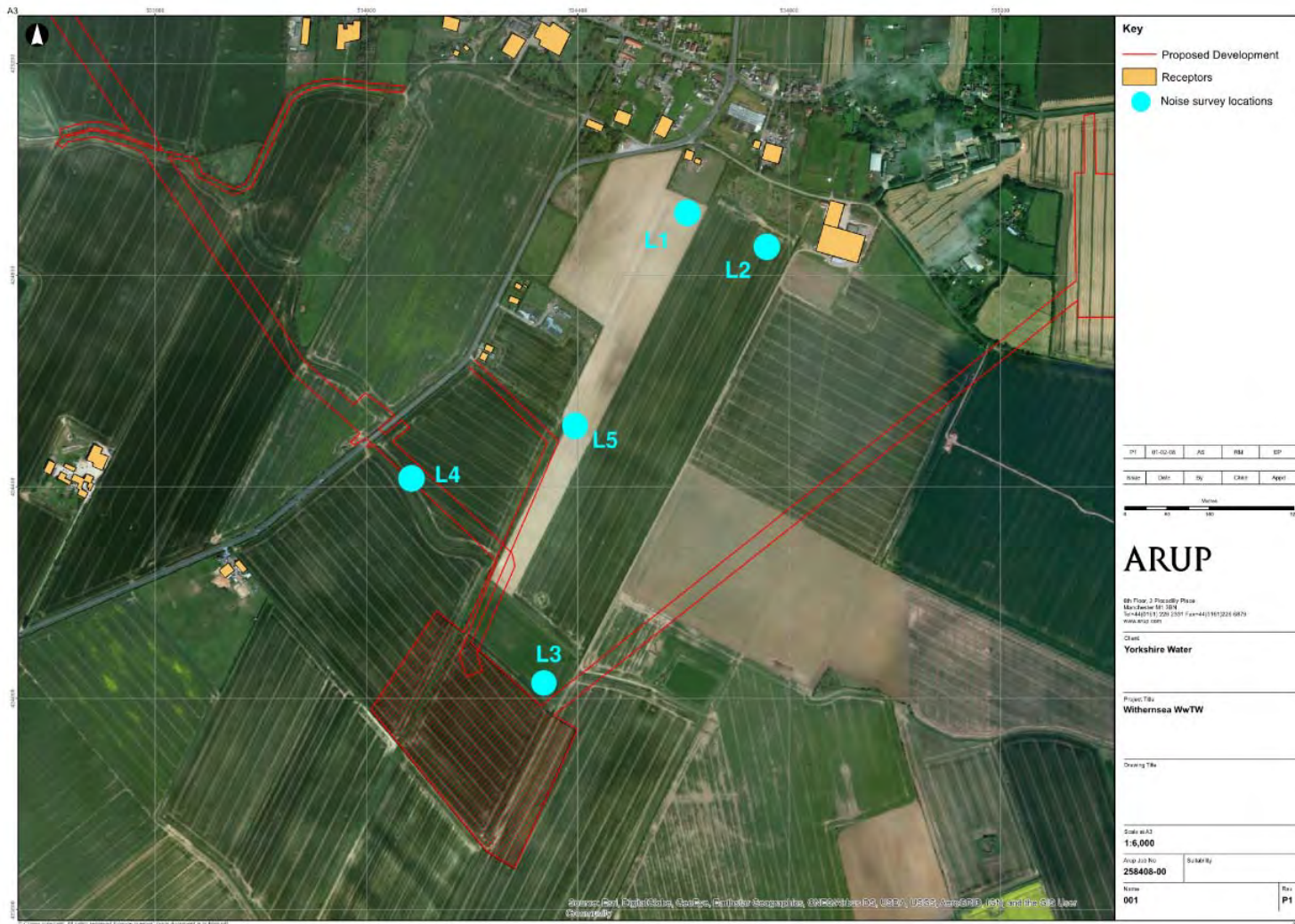
Figure 2: Noise measurement locations (the indicative WwTW site boundary is shaded in red- please see drawing 41522050_01_G_0701 for formal red line boundary)
